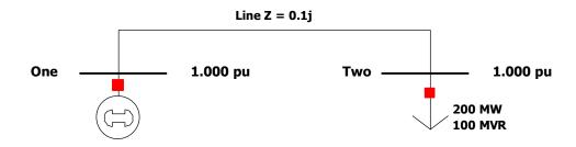
For the system above, find the Y-bus matrix. (The transmission line does not have any resistance or capacitance modeled, and loads and generators are not generally part of the Y-bus matrix.)
