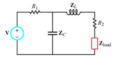
Second order transient. Determine  $v_{\mathcal{C}}(t)$  for t > 0.
