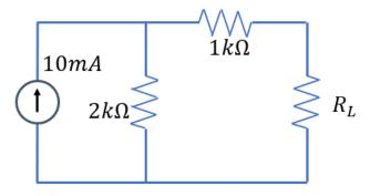
40. What's the maximum power that can be delivered to the load resistor  $R_L$ ?
