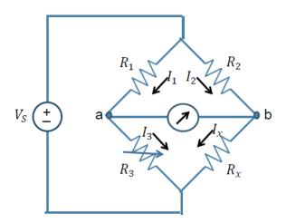
For the Wheatstone bridge circuit above, we have  $R_1 = 5\Omega$ ,  $R_2 = 20k\Omega$ .  $R_3$  is a variable resistor between 0 and 100  $\Omega$  that we adjust until the Ammeter shows 0 A.
