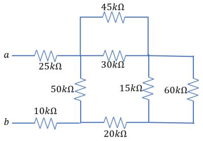
33. What is the equivalent resistance between a and b in the below circuit?
