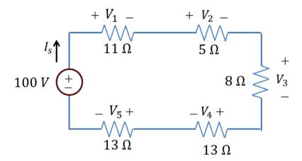
Solve for  $I_s$  and the current through each resistor
